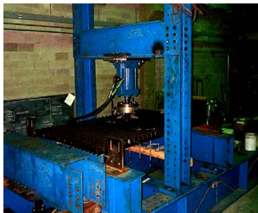
Figure 4.1 – Load Frame and Weldless Deck
